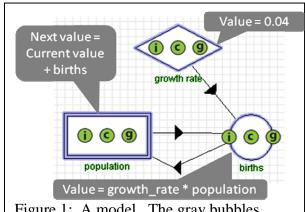
Figure 1: A model. The gray bubbles, which are not normally visible, show how the value of each variable is calculated.
