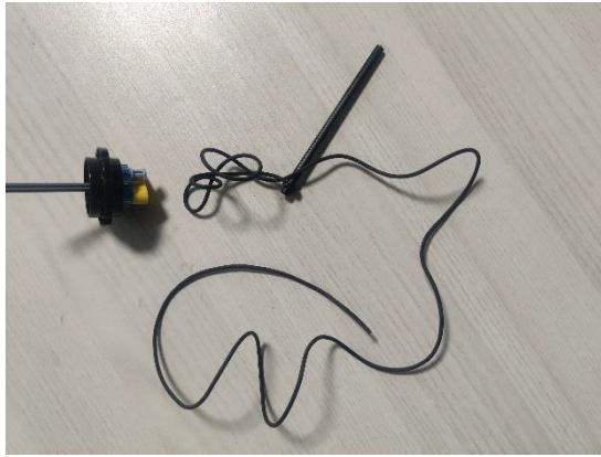
Figure 1. The earphone wire – lego components combination for supporting the gripper movement.
