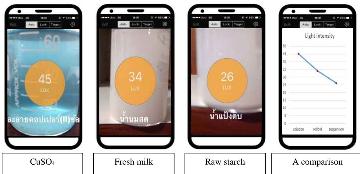
Figure 2. Illustrations of smartphone screen in measuring the intensity of light passing through solutions, suspensions, and colloids, a comparison graph
