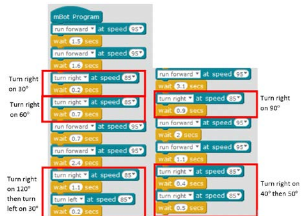
Figure 1(b). An example that illustrates the sequencing ability of students by auto-piloting a robotic car to run a square with codes not in a generalizable pattern.
