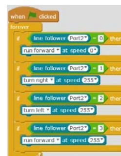
Figure 3(b). An example of a piece of codes illustrating implementation of conditional reasoning in piloting a robotic car to run along the white track.
