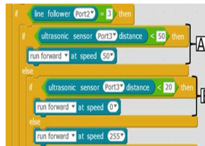
Figure 4. An example illustrating the ability of systems thinking of students in auto-piloting a robotic car to move along the white track and additionally need to slow down and stop when an obstacle is detected.
