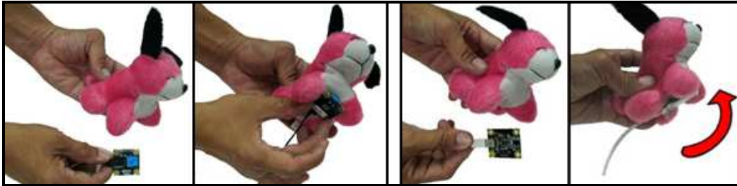
Fig. 6. Force sensor and spatial sensor glued on tangible object in TangiLearn
