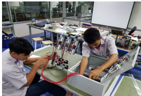
Figure 4. Pneumatic control project with relay circuit.
