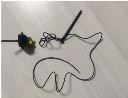
Figure 3. The earphone wire – lego components combination for supporting the gripper movement.
