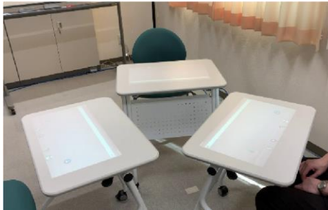
Figure 2. An example of UI projection for three desks separately, using one projector & one sensor.
