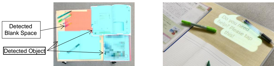
Figure 4. An example detection result on a desk*. Figure 5. An example of projected adaptive UI*.
