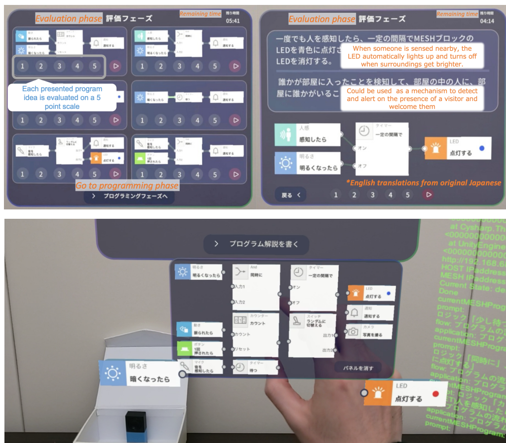
Figure 3. Top : The evaluation phase interface, where users can view and provide feedback on MESH programs created by other users or generated by the system. Bottom : The programming phase interface, where users can create MESH programs by connecting virtual MESH blocks in an AR environment.
