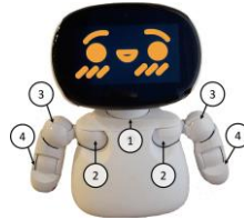
Figure 1. Kebbi is equipped with seven motors that govern different components of its body. These components include a neck (1), two shoulders (2), two elbows (3), and two fists (4).
