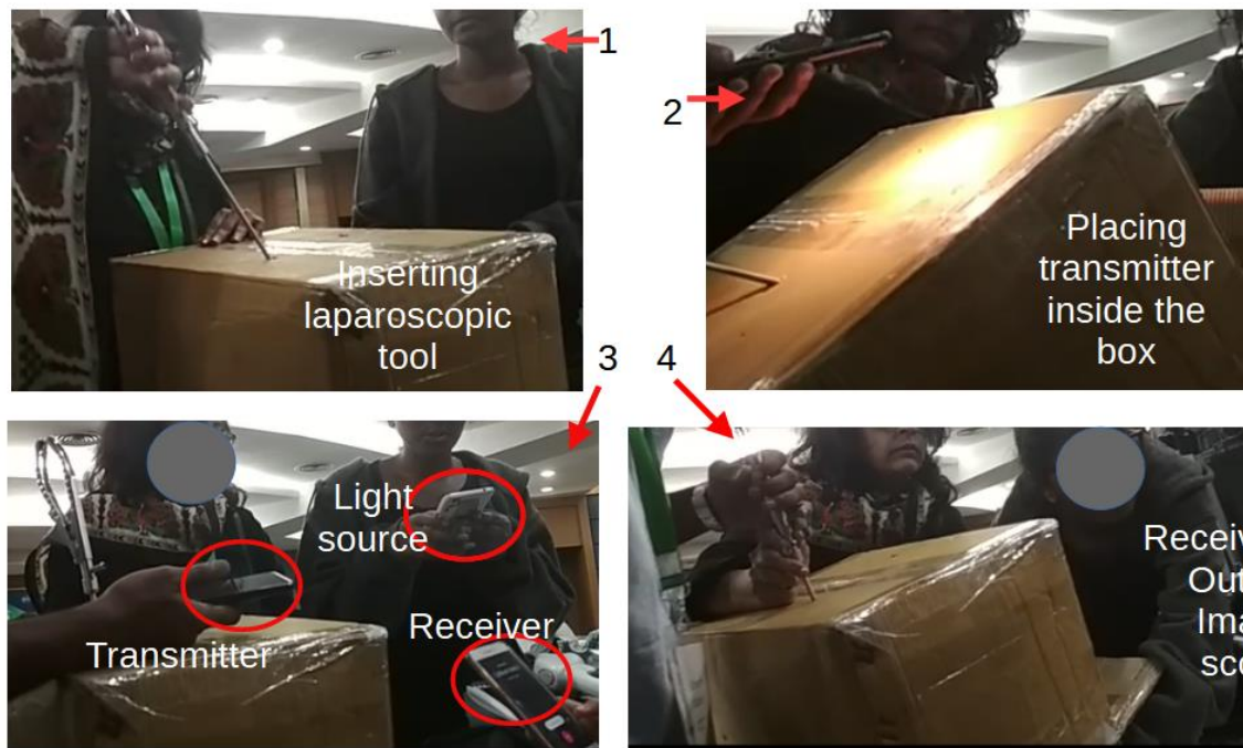
Steps to simulating the laparoscopic suturing process using 3 mobiles, cardboard box as the human body and the laparoscopic tools.
