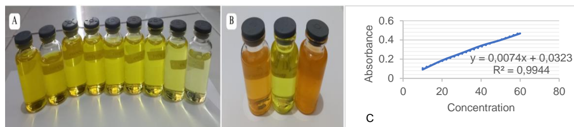
Figure 4. (A) Standard tartrazine solution (B) Sample solutions from 3 different brands of beverages (C) Graph of the Relationship between Absorbance and Concentration of Standard Tartrazine Solution
