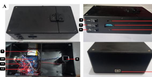
Figure 2. (A) Simple Spectrophotometer Instrument Side and Top View
