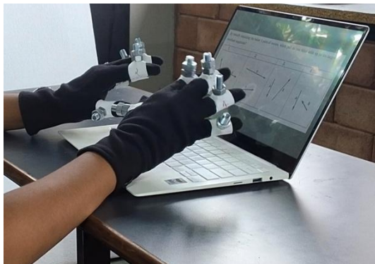
Figure 1. Experimental setup for Experiment 1 (Finger Weights). (a) Weighted condition: participants wore gloves with elastic bands fitted with nuts and bolts on the thumb, index, and middle fingers ( \approx 170 g total). (b) Control condition: participants wore identical gloves with elastic bands but without added weights. This ensured that tactile sensation and movement restriction were comparable across groups.
