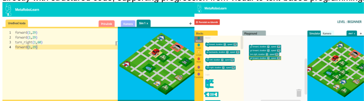
Figure 2. Equivalent robot program implemented in Python (left) and Blockly (right).
