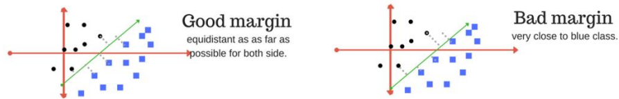
Figure 3: Types of margins, good margin and bad margin Source: self made.
